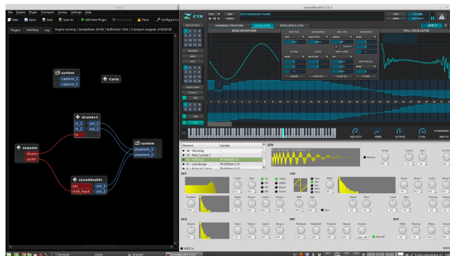
Figure 1: A Sequoia session is connected to two different client applications using JACK. Here ZynAddSubFX ( zyn-fusion ) and drumkv1 are being used to create a simple beat. Carla is used to manage audio and MIDI connections.
