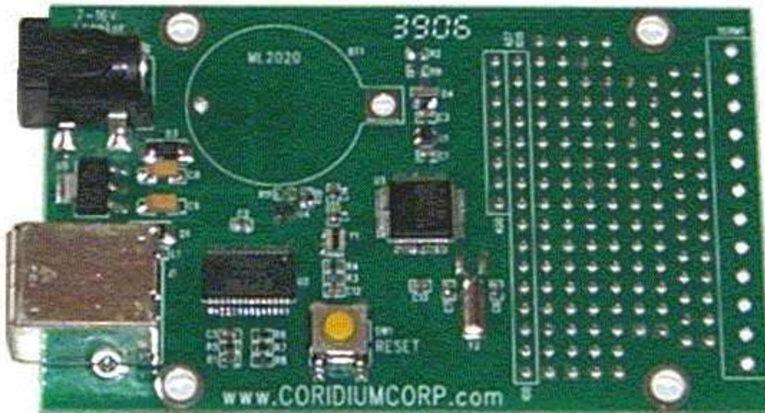
The timing resolution is 1 $\mu$ s, way above what we need here. The board can be programmed in Basic. The firmware for this board can be downloaded freely for examination: [Arm\\_Midi\\_PIR2.bas](#). The data channel scan rate we found suitable is 25S/s. The data rate for our applications leads to a
