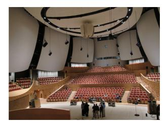
We had not tested the system in an enclosed environment, and needed to verify that we could achieve the wet signal energy of Hagia Sophia without feedback. Using a group of seven Byzantine chanters from the choir of Holy Cross Church in Belmont, we were able to produce the needed levels of reverberation without feedback, provided head-mounted microphones were used.
