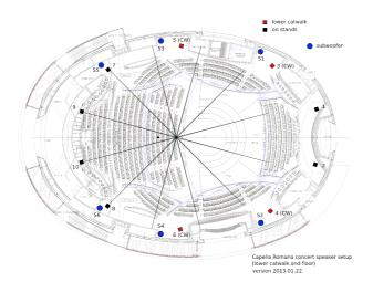
The speakers rigged from the ceiling were roughly arranged in two "rings", a medium height one comprised of 10 speakers and a high ring of four speakers. The placement of the speakers was restricted by the spacing and availability of rigging points so it is not an exactly regular arrangement.
