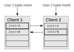
Figure 2: Instrument synchronization
