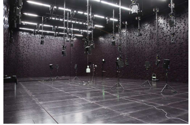
Figure 5: Speaker rig and measurement setup at Ligeti Hall in MUMUTH Graz
