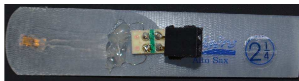
Figure 1: Synthetic alto-saxophone reed with 2 mm strain gauge attached
