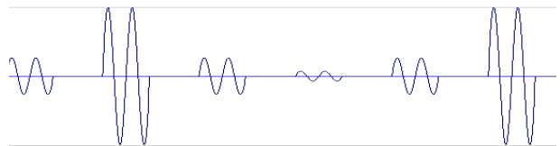
Figure 6: Amplitude masked pulsar train
